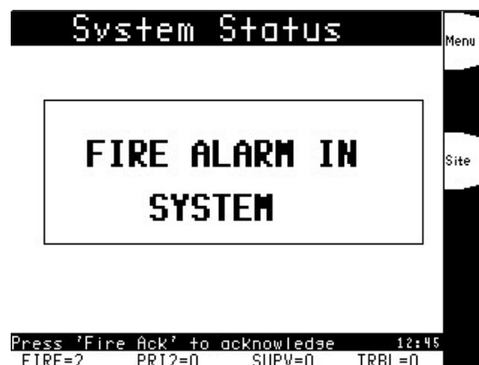
Figure 8: General Alarm Primary Display Option
