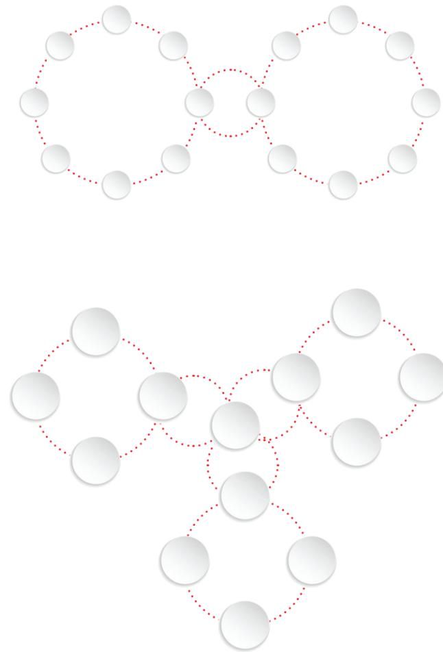
ES Net eases design and installation by supporting ring, star, bus and bridged ring network topologies. Because you can combine multiple topologies, you can create fault-tolerant, highly survivable networks while mixing and matching media between nodes to optimize cost, distances and performance.
